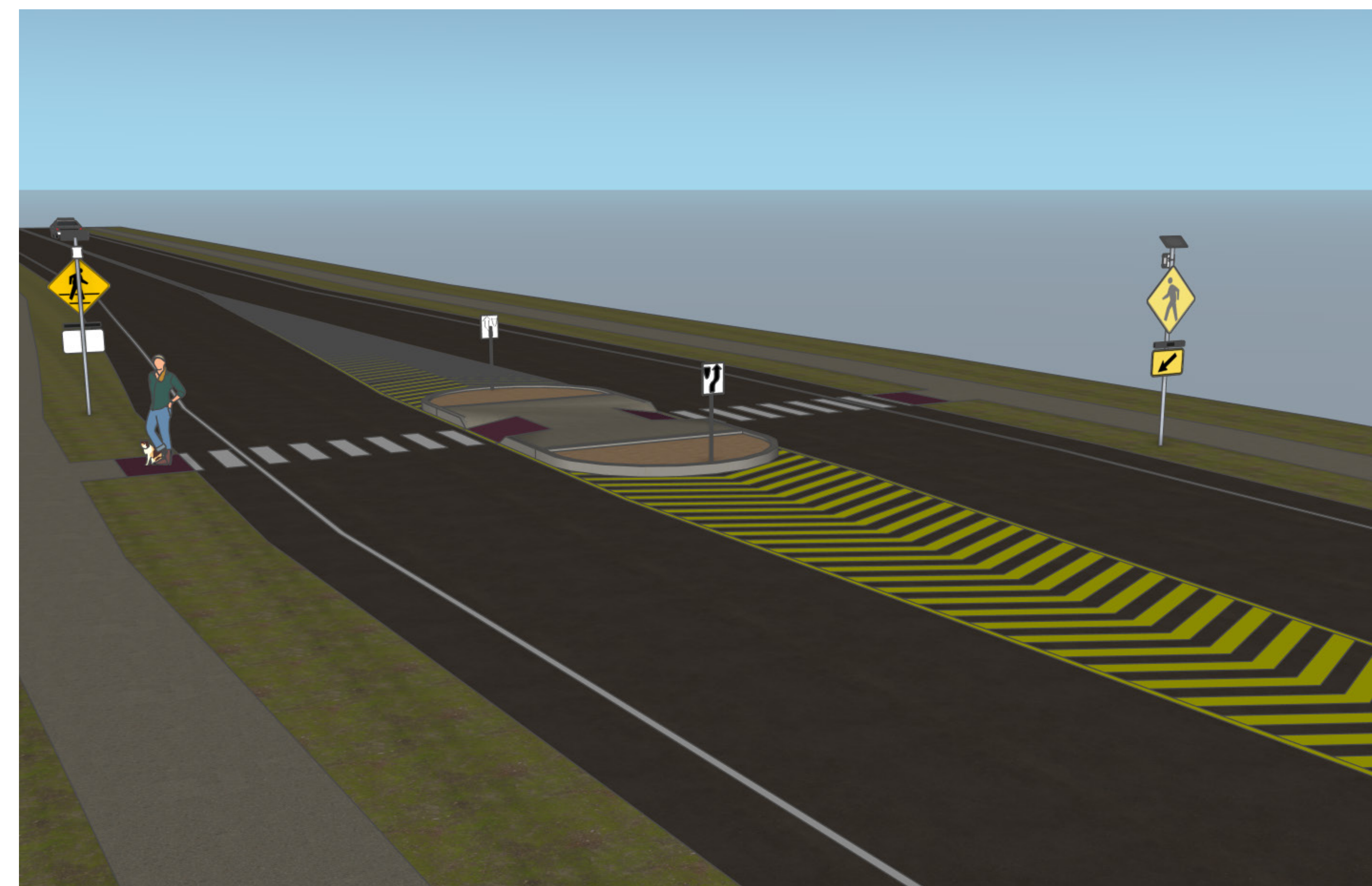
Crosswalk with refuge island and RRFB signage.
