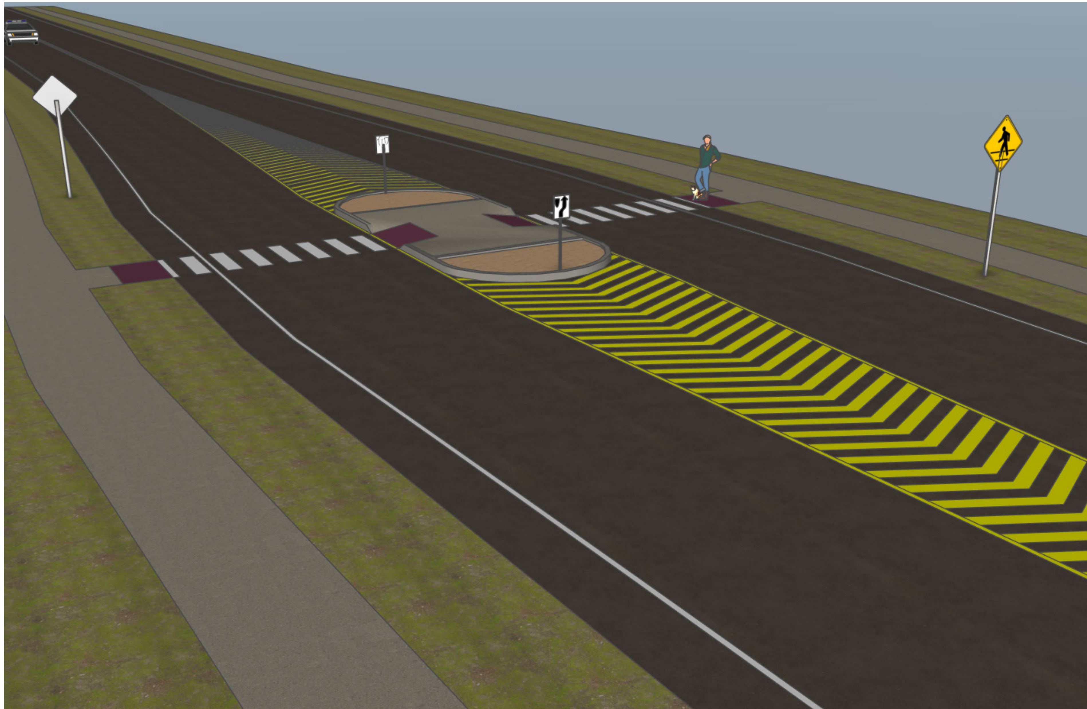
Crosswalk with refuge island and standard signage.
