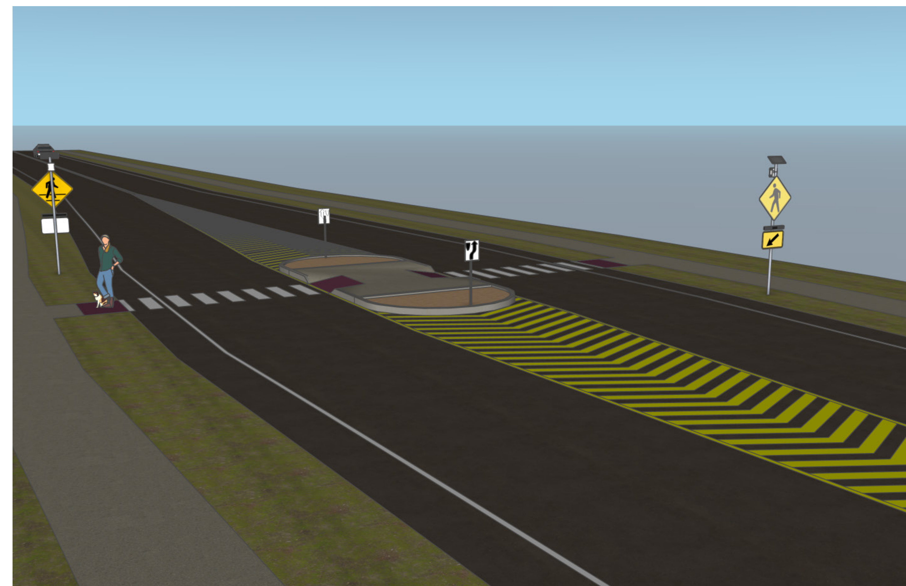
Crosswalk with refuge island and RRFB signage.
