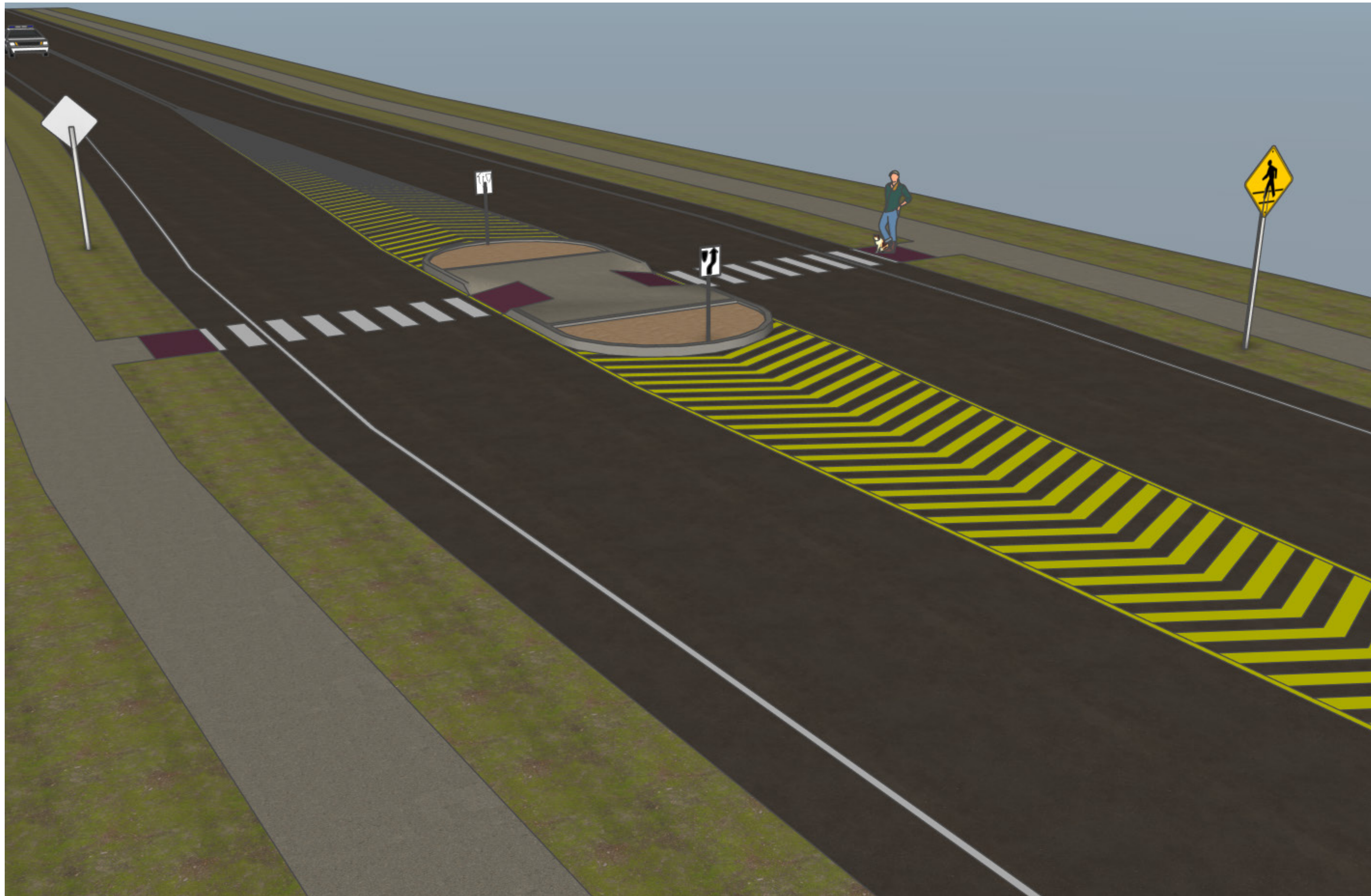
Crosswalk with refuge island and standard signage.
