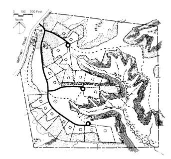
Figure 18 STEP FOUR Drawing in the Lot Lines
