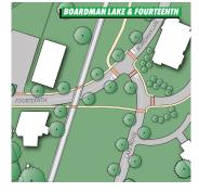
Boardman Lake & Fourteenth It is recommended that Boardman Lake Avenue be extended to connect to Fourteenth to increase connectivity and relieve Cass as the north/south connector. A T-Intersection is recommended to accommodate Lake Ridge while still providing for an efficient flow of traffic from Boardman Lake Avenue to Fourteenth. 500 feet
