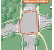
Division & Fourteenth If a roundabout does not prove feasible, it is recommended that the City build upon the existing signal configuration of the intersection at Division and Fourteenth to include two left turn lanes, a through and a through-right lane for westbound traffic and a left turn, a through, and right turn lane for eastbound traffic. The eastbound, northbound and southbound configurations should incorporate an additional through-lane to support increasing traffic patterns.
