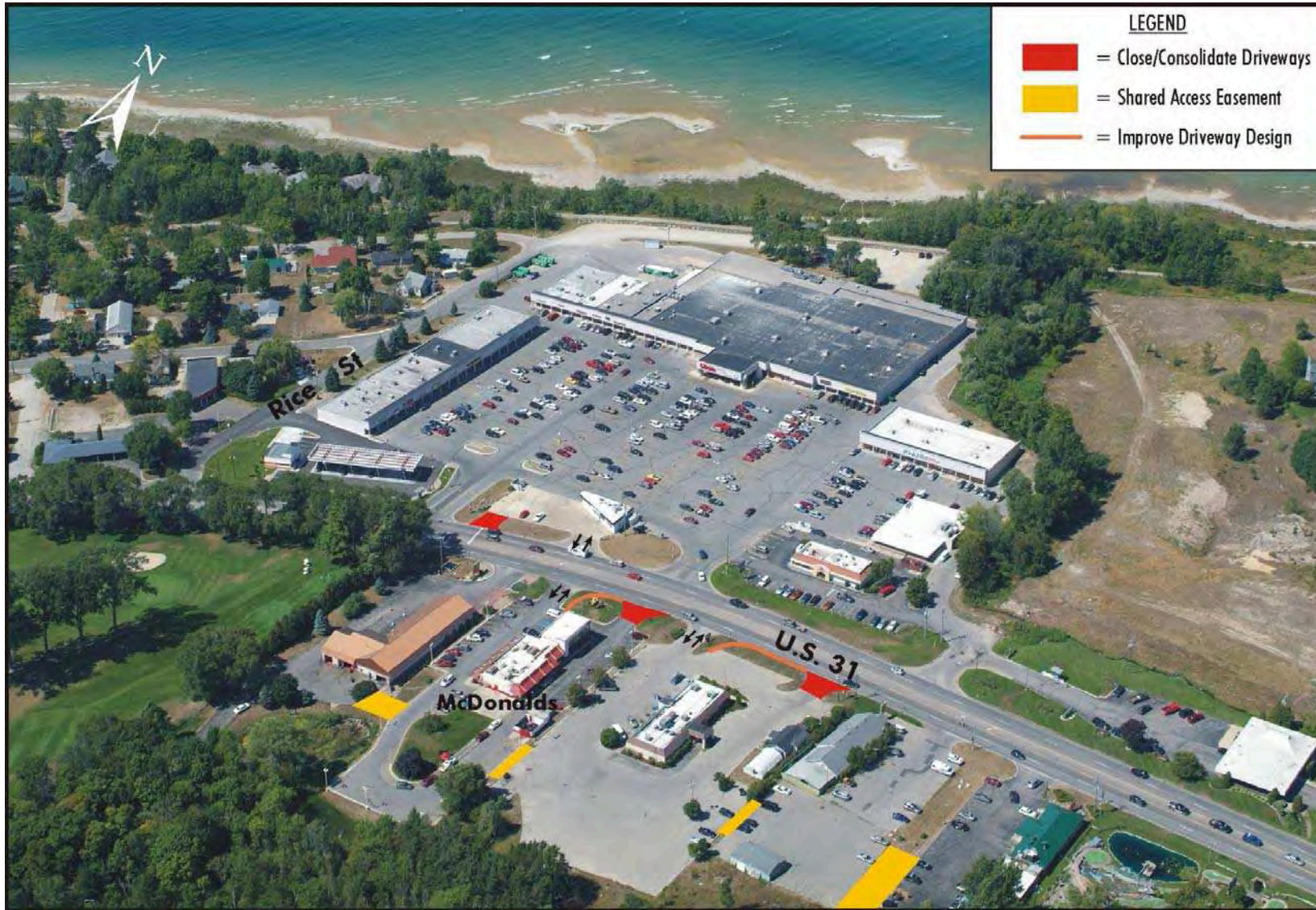
Figure 3-25 Petoskey Area-wide Transportation Concepts Access Management Concepts in Area of U.S. 31 and Rice Street
