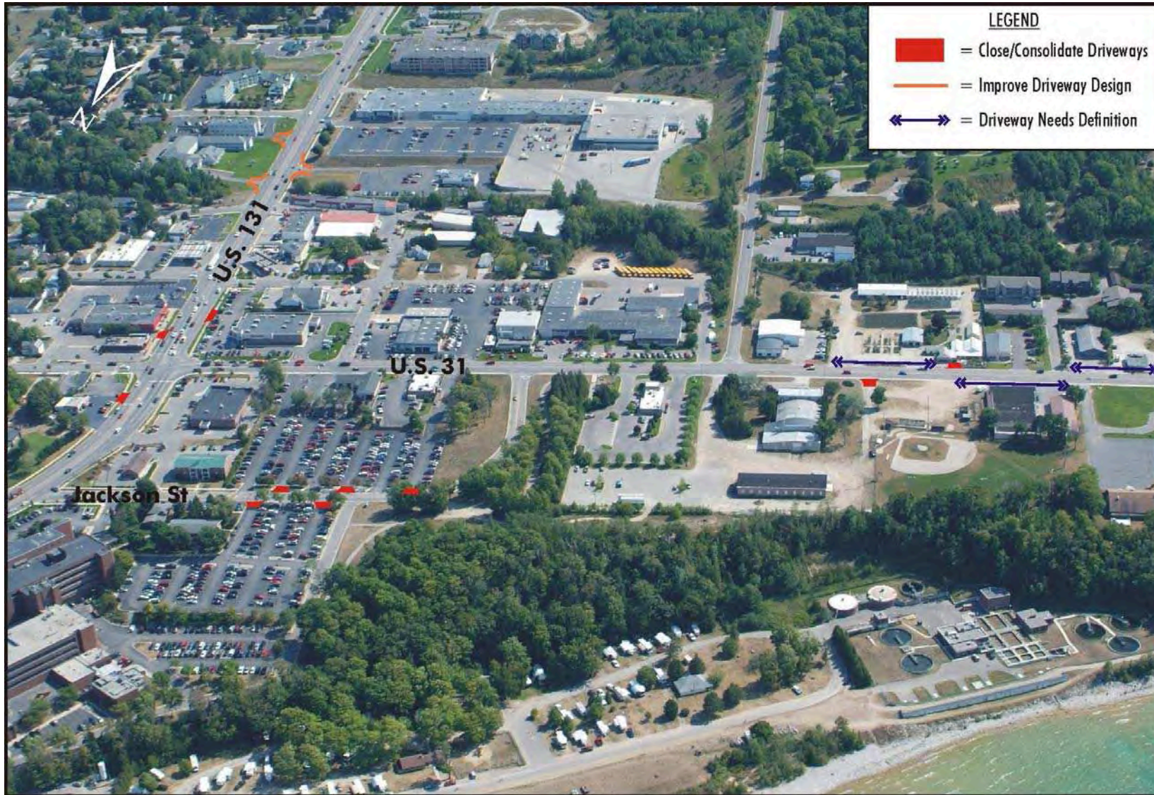
Figure 3-27 Petoskey Area-wide Transportation Concepts Access Management Concepts in Area of U.S. 31 and U.S. 131
